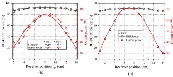
**Fig. 14.** Performance variation against asymmetric misalignment for the (a) receiver movement in  $y$ -direction (i.e., Case D and Case E) and (b) receiver movement in the diagonal direction (i.e., Case F).
