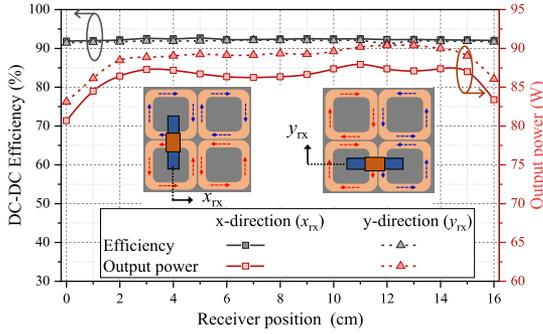
Fig. 10. Variation of the output power and efficiency with respect to the receiver movement in the  $x$ - and  $y$ -directions.
