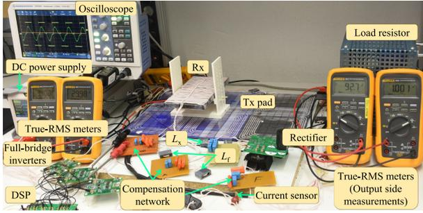
Fig. 5. Experimental setup.
