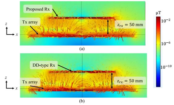
Fig. 4. Distribution of magnetic flux density of a four-Tx WPT system: Front view in the  $xz$ -plane at  $y = 0$  (magnetic field vectors are shown with arrows), for (a) proposed receiver type and (b) classical DD-type receiver.
