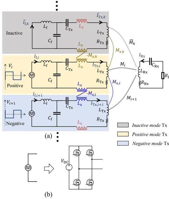
Fig. 2. (a) Equivalent circuit of a multi-Tx WPT system with *positive* mode, *negative* mode, and *inactive* Tx. (b) Illustration of a full-bridge inverter as the power source.
