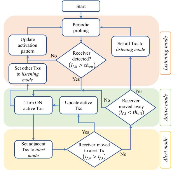
Fig. 6. Flowchart of the proposed Tx activation/deactivation.
