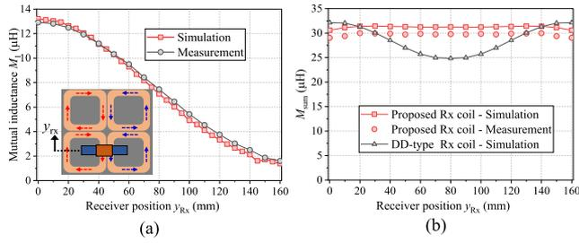
Fig. 3. (a) Simulated and measured mutual inductances between a single Tx ( $T_{x1}$ ) and Rx with respect to the variation of the receiver position in  $y$ -direction ( $y_{Rx}$ ). (b)  $M_{sum}$  variation of the proposed flux-pipe type receiver is compared with conventional DD-type receiver with the same dimensions and number of turns.
