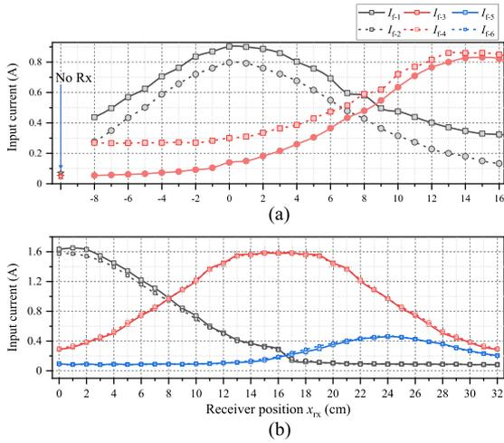
Fig. 7. Input current of the active and inactive Tx coils.
