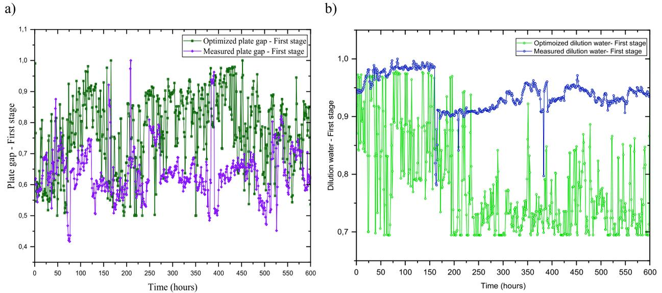
Figure 13: Representative normalized optimum and measured values for first-stage a) refining plate gap, and b) refining dilution water.
