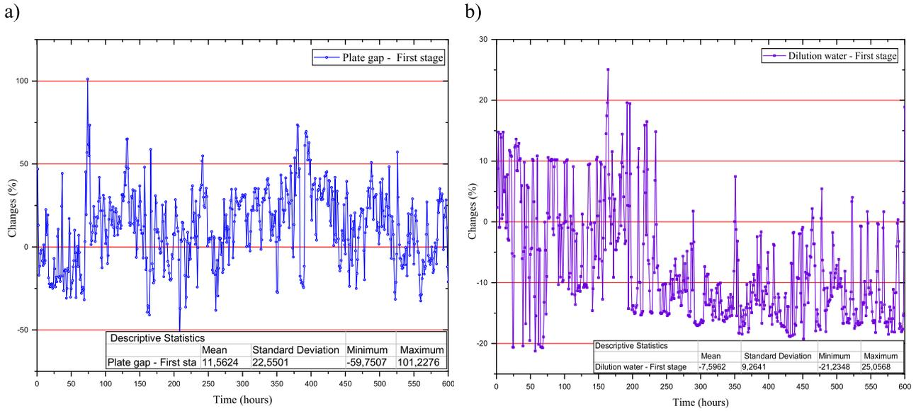
**Figure 15:** Representative percentages of change in the first-stage a) plate gap and b) dilution water from the measured value to the optimized value (the calculation term is explained in Equation 14).
