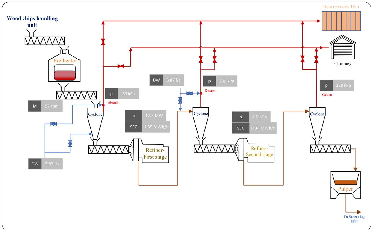
Figure 2: Schematic of the main refining line with sample measured data.
