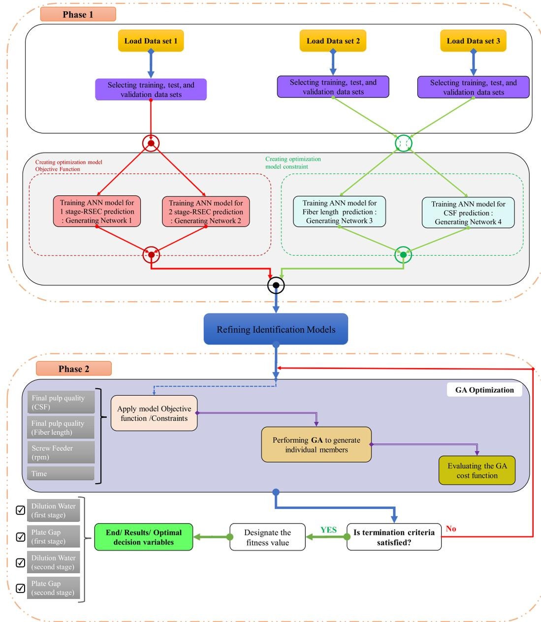
Figure 6: Schematic representation of the proposed advanced energy-saving refining optimization strategy.
