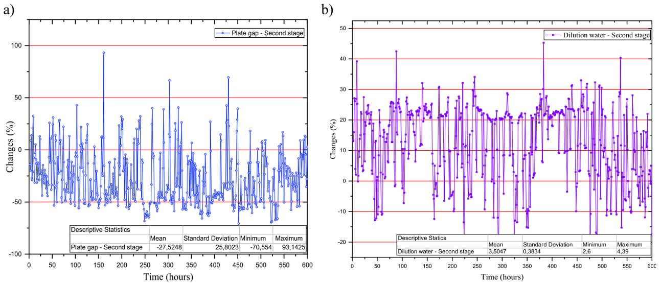
**Figure 16:** Representative percentages of change in the second-stage a) plate gap and b) dilution water from the measured value to the optimized value (the calculation term is explained in Equation 14).
