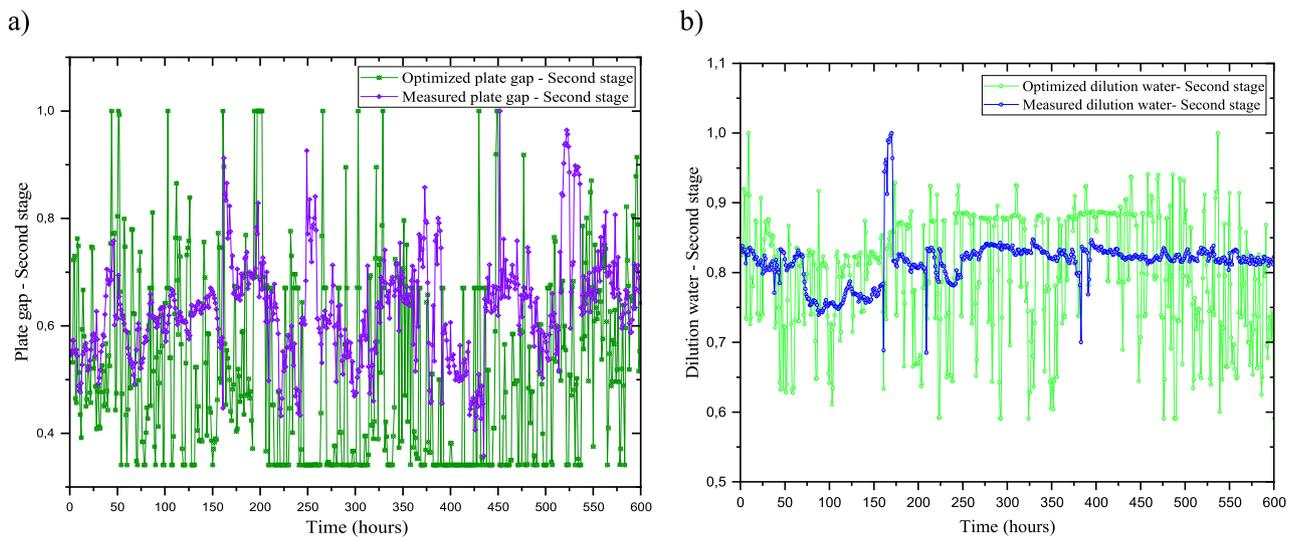
Figure 14: Representative normalized optimum and measured values for second-stage a) refining plate gap, and b) refining dilution water.
