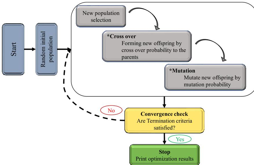
Figure 4: The design structure of the genetic algorithm.
