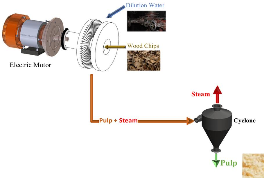
Figure 1: Mechanical refining principle.
