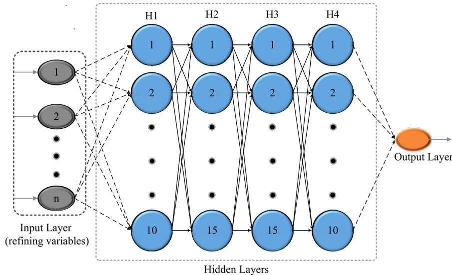
Figure 5: The architecture representation of the optimum ANN consists of four hidden layers.
