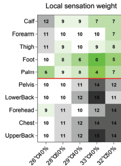
Fig. 3. Weight coefficients (%) of local thermal sensation on overall thermal sensation under different conditions.
