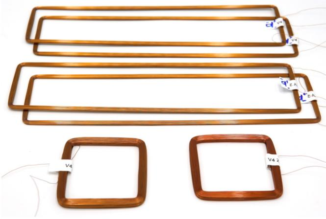
Fig. 13. In-house manufactured magnetorquers.
