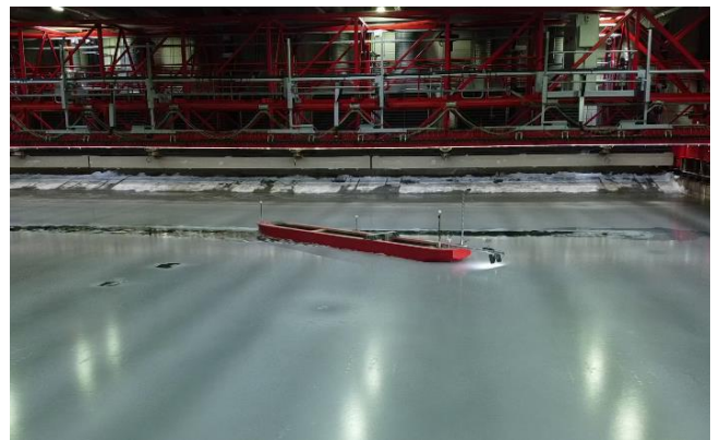
Figure 3. Model ship Infuture breaking out of channel
