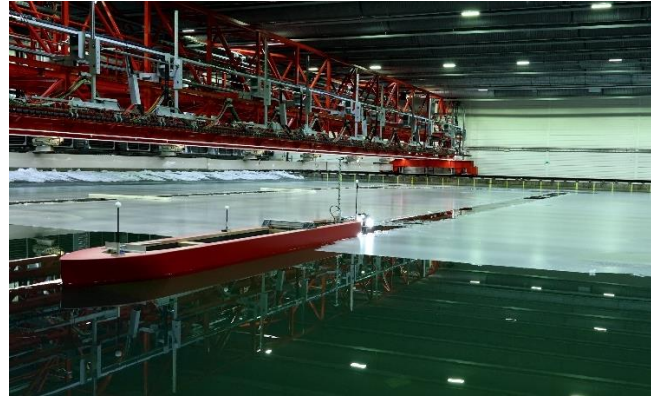
Figure 2. Model ship and ice channel before breakout test starts
