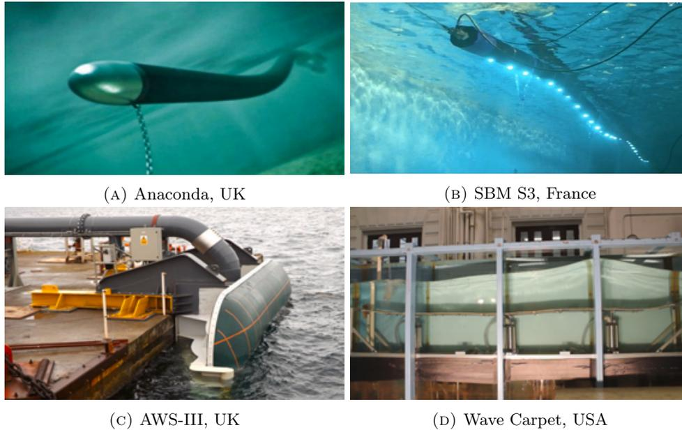
FIGURE 15. Flexible WECs: existing examples
