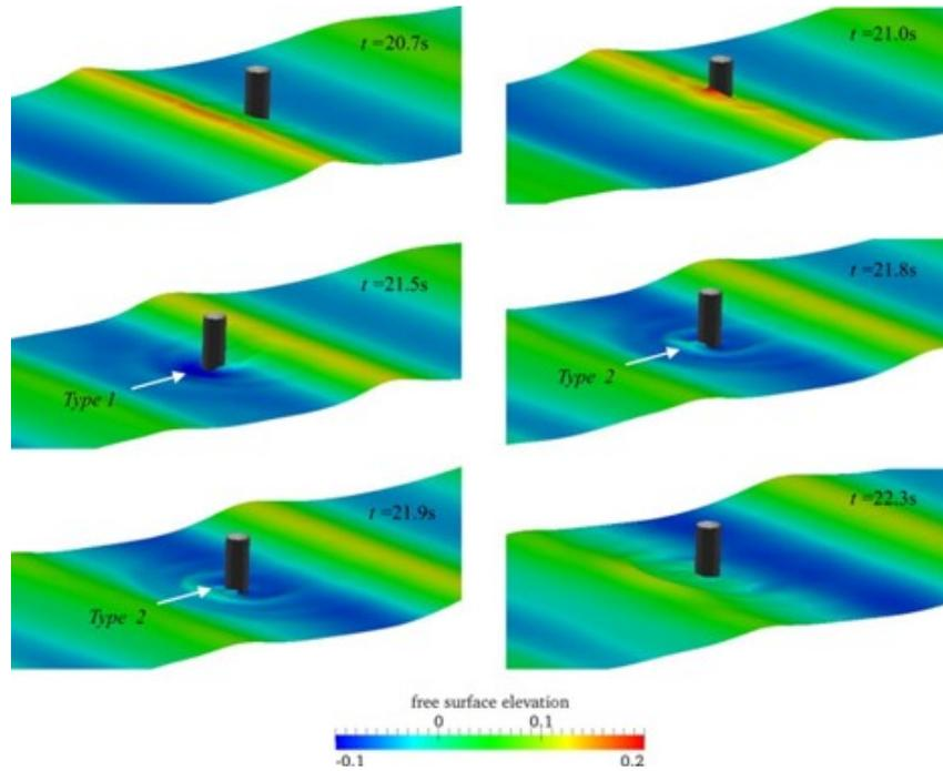
FIGURE 8. Uni-directional waves interacting with a fixed cylinder [41]
