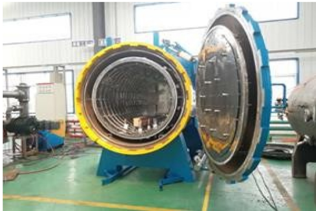
Fig. 6 – Vacuum sintering plant [116].
