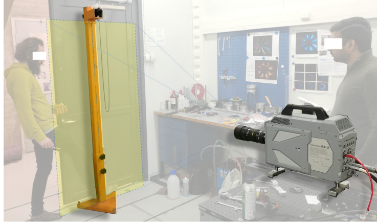
Fig. 2. The experimental set-up with the high speed camera (Photron SA-Z) and the folded chain in its initial configuration.
