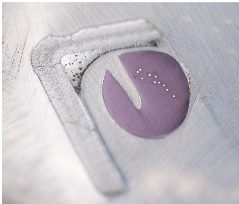
Figure 1. Photograph of a typical sample cross-section in epoxy after analyses. The violet color of the copper alloy is a result of carbon coating. The small holes on the slag and copper alloy are laser pits produced by LA-ICP-MS. Photo: Aalto University, Eren Öztekin.
