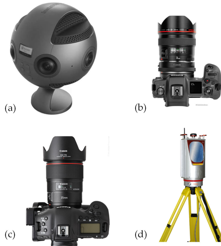
Figure 3. Hardware used in this study: (a) Insta360 Pro with 6 fisheye lenses, (b) Canon EOS RP mirrorless DSLR with 14 mm lens to capture the reference DSLR model, (c) Canon 5Ds R DSLR with 35 mm lens to capture the High-Quality images for the improved 360 + HQ model, and (d) Riegl VZ-400i terrestrial laser scanner.
