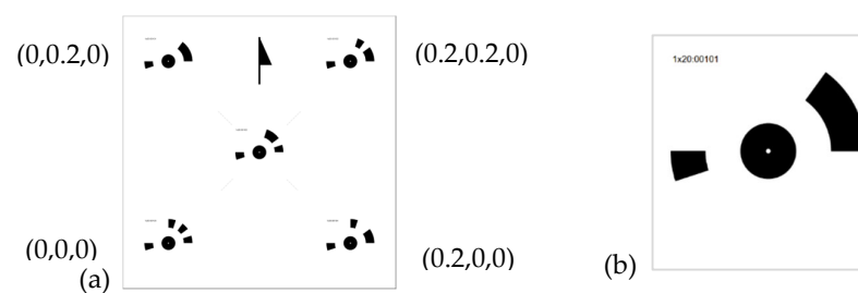
Figure 2. Orientation control board (a) with known local coordinates used to orient the 3D model, and (b) control point example that was used in the field test to control the accuracy of SfM-MVS reconstruction.
