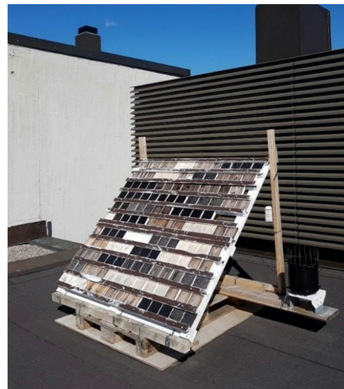
Fig. 1 Left: Relative humidity (%), monthly rainfall (mm) and averages of monthly temperature (°C); Right: The weathering rack after three months of weathering in September 2020
