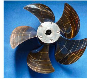
Fig. 2. Photograph of the PPTC propeller.
