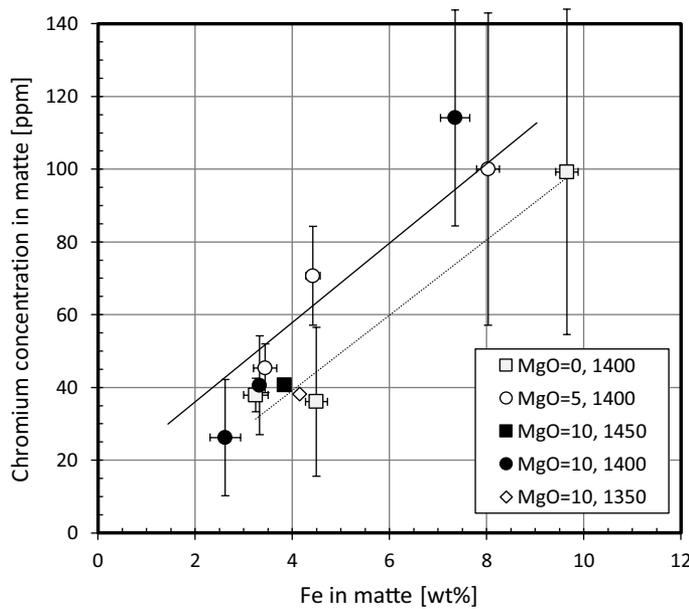
**Figure 4.** Measured solubilities of chromium in nickel mattes at 1350–1450°C analyzed by LA-HR-ICP-MS as a function of iron concentration of the DON matte analyzed by EPMA; symbols refer to various MgO concentrations of the slag (--- MgO = 0, - MgO = 5,10 wt%).
