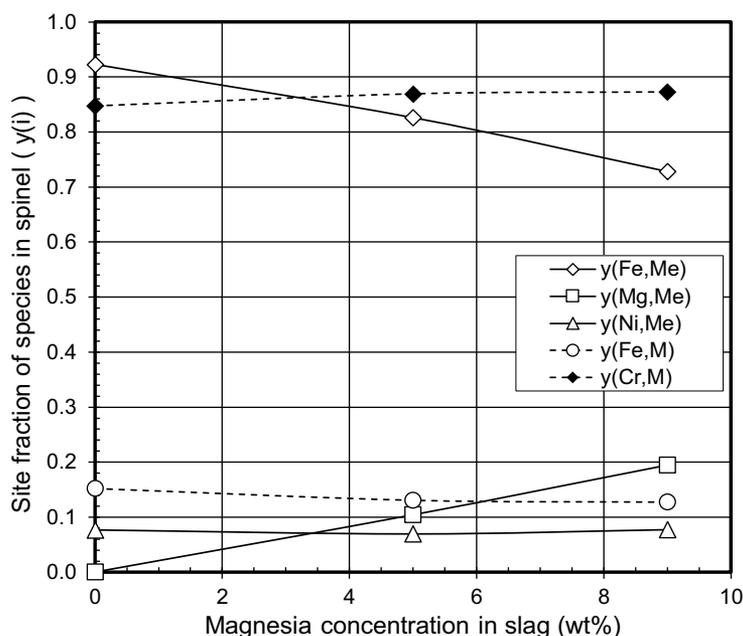
**Figure 6.** The estimated distributions of cations in the spinel  $(Me)(M)_2(O)_4$  sublattices as a function of magnesia concentration of the bulk slag at silica-spinel saturation at 1400°C.
