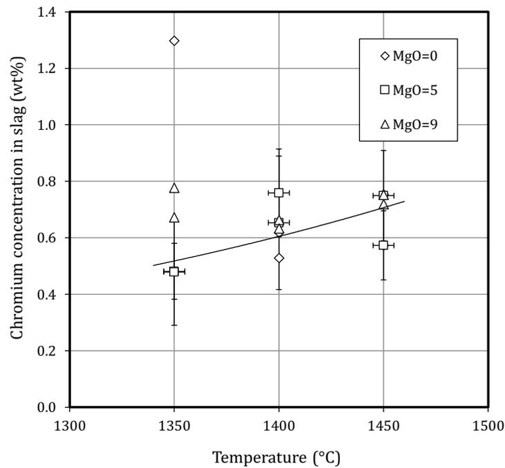
**Figure 2.** The impact of temperature on the chromium solubility in silica-spinel saturated, molten iron-silicate slags at 1350–1450°C and 5 wt% [Fe] in the DON matte; the trend line has been fitted to the points with 5 wt% (MgO).
