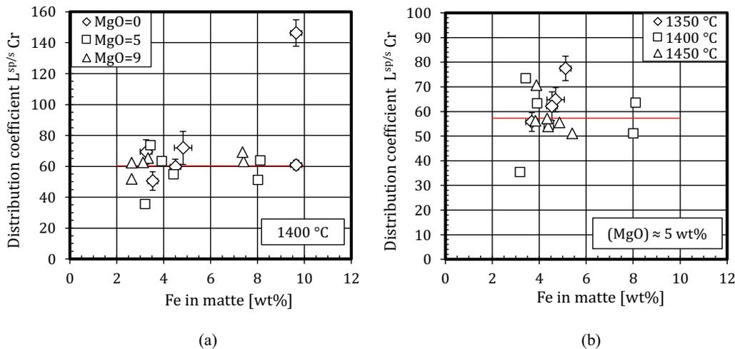
**Figure 3.** Distribution coefficient of chromium between spinel and molten slag (a) at 1400°C as a function of the iron concentration of the DON matte and (b) at 5 wt% MgO in the slag at 1350–1450°C; the error bars in (a) refer to the experimental data at 0 wt% MgO in the slag and in (b) at 1350°C. The red horizontal lines show the average of the experimental points presented in each diagram.
