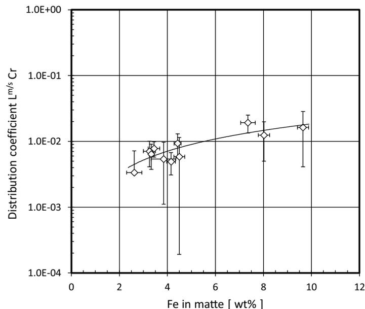
**Figure 5.** The distribution coefficient of chromium between nickel matte and iron-silicate slag at 1350–1450°C as a function of iron concentration of the DON matte; the various MgO concentrations of the slag cannot be distinguished from each other due to scattering in the distribution coefficient values.
