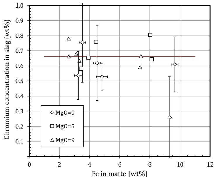
**Figure 1.** The obtained solubilities of chromium in molten iron-silicate slags at silica-spinel saturation as a function of iron concentration of nickel matte at 1400°C; the error bars show the standard deviations of the results with MgO = 0 in the slag and the red horizontal line shows the average value of all experimental points of 0.66 wt % (Cr).
