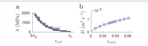
**Fig. 2 a** The strain evolution of the expected average hardening coefficient  $\langle h \rangle$  (blue) and the local hardening parameter values from one simulation (grey). The drops in the local hardening coefficient signify increases in the local plastic strain due to passing of bands. **b** The strain rate dependence of the parameter  $D = D_0 \epsilon_{ext}^{\nu}$
