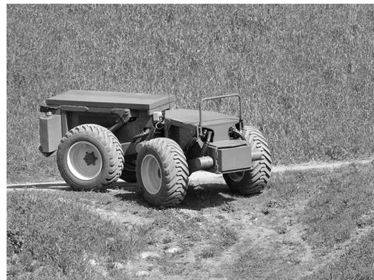
Fig. 1. A photograph of the Rakkatec unmanned ground vehicle (Rakka-UGV). The vehicle can be seen maneuvering using center-articulated steering (courtesy: Rakkatec Ltd.).
