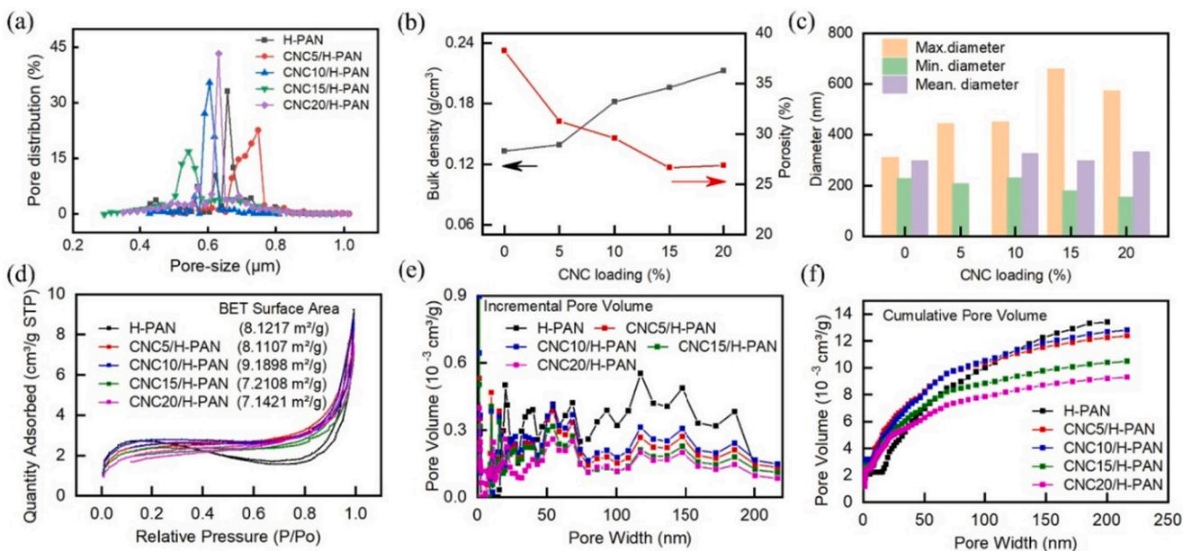
**Fig. 4.** (a) Pore size distribution (PSD) profile of CNC/H-PAN ENMs obtained by the bubble point method, and (b, c) physical properties of the nanofibers and membrane structure. (d)  $N_2$  adsorption–desorption isotherm of membranes (e, f) Pore size distribution (PSD) curve calculated by DFT method according to  $N_2$  adsorption–desorption isotherm. (For interpretation of the references to color in this figure legend, the reader is referred to the web version of this article.)
