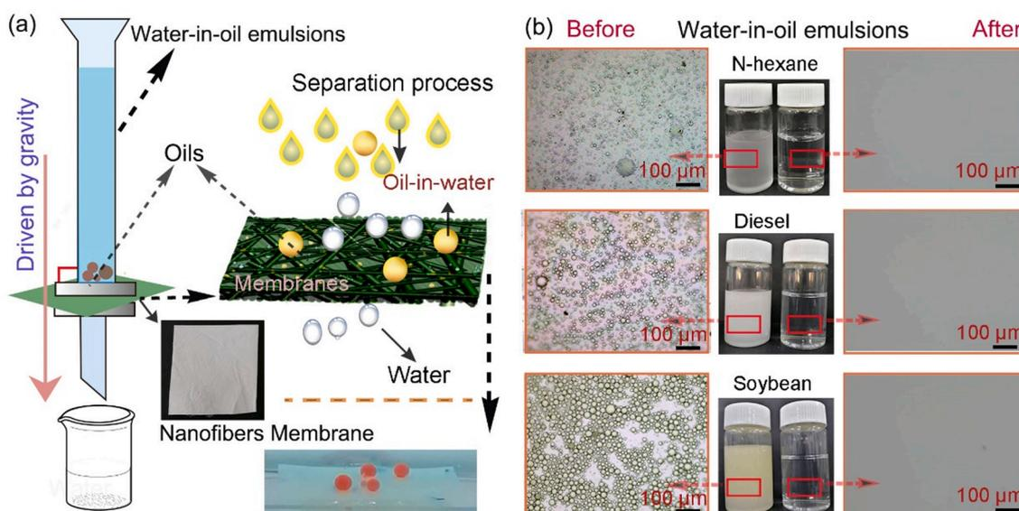
Fig. 6. (a) Schematic diagram of O/W emulsions separation process (b) Optical microscope image of O/W emulsion before (left) and after filtration (right for the filtrate). (For interpretation of the references to color in this figure legend, the reader is referred to the web version of this article.)
