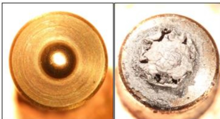
Fig. 11. Injector tip before cycle (left cycle) and after cycle (right side)
