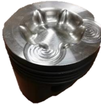
Fig. 3. High compression ratio (CR = 22:1) wave piston
