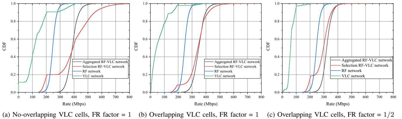
Fig. 4: Effect of the integration approaches on the user data rate in case of different multi-cell VLC configurations. No overlapping ( $\Psi_{\max} = 45^\circ$ ) vs. moderate overlapping ( $\Psi_{\max} = 60^\circ$ ). High FR factor (FR = 1) vs. moderate (FR = 1/2).
