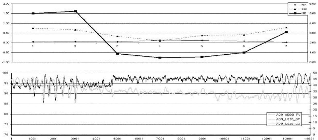
Fig. 2. Performance indices for the loop describing normal controller behavior
