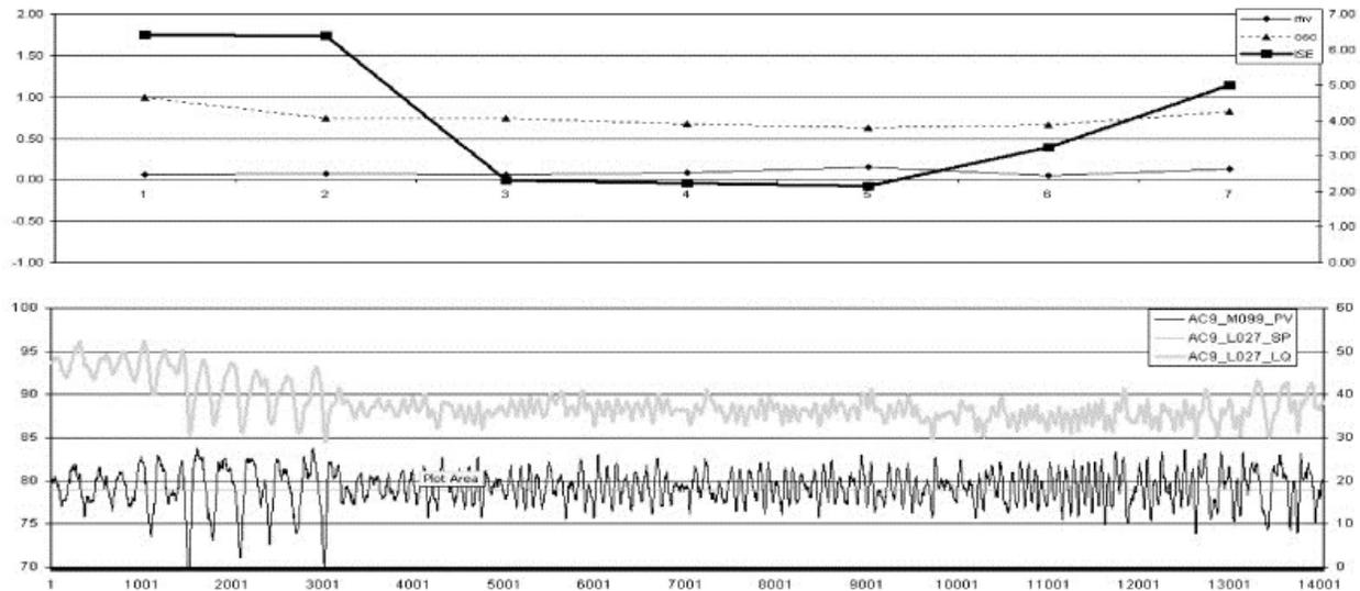
Fig. 3. Performance indices for the loop describing oscillating controller behavior
