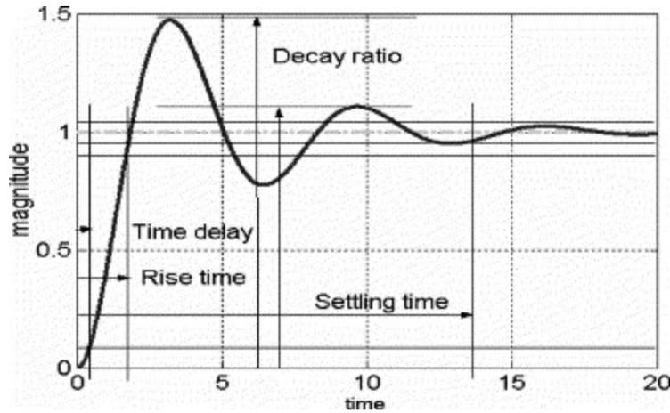
**Fig. 1.** Response to a step change in a set-point
