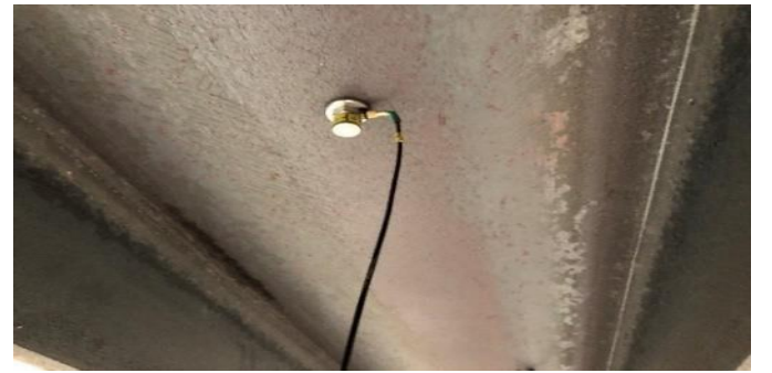
(b) Installation of the accelerometer.
