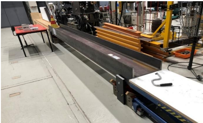
Figure 2. Steel beam used as a bridge model.
