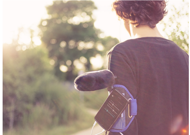
Figure 1. The final version of Wandertroper being worn on the arm. The armband allows the device to be positioned and oriented in different ways. These influence the mobile sensors, which affect how the sound is manipulated. The external microphone was optional, and was often not used in practice.
