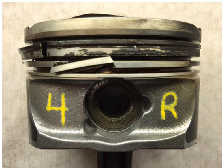
Fig. 10. Damage caused by super-knock to piston ring lands.
