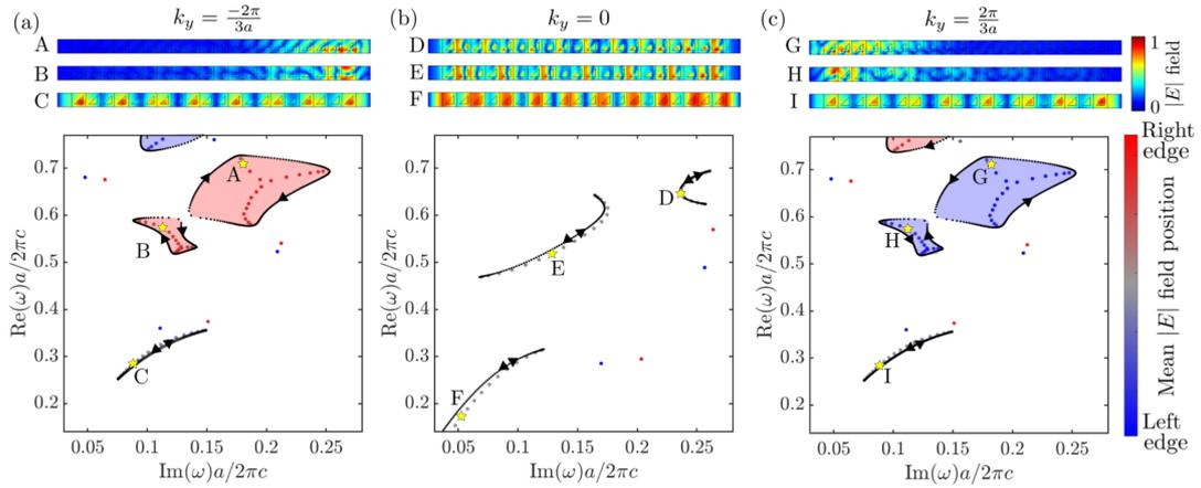
Fig. 2. The lower part of each panel shows the complex band structure of the infinite 2D photonic crystal in solid black, where arrows give the direction of winding. The red and blue dots are the eigenfrequencies of the finite stripe geometry. (a), (b) and (c) correspond to  $k_y = \frac{-2\pi}{3a}, 0$  and  $k_y = \frac{2\pi}{3a}$  respectively and A-I are the normalized electric field eigenstates which show the skin effect.
