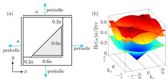
Fig. 1. (a) Unit cell of photonic crystal where the lattice periodicity is  $a$ . Here, the background is air and the triangle has refractive index  $n_{\text{tri}} = 2 - 1i$ . (b) The lowest three bands of the real part of the eigenfrequencies in the first Brillouin zone for the photonic crystal geometry in (a). The dashed black lines are at fixed  $k_y = -\frac{2\pi}{3a}, 0$  and  $\frac{2\pi}{3a}$ .
