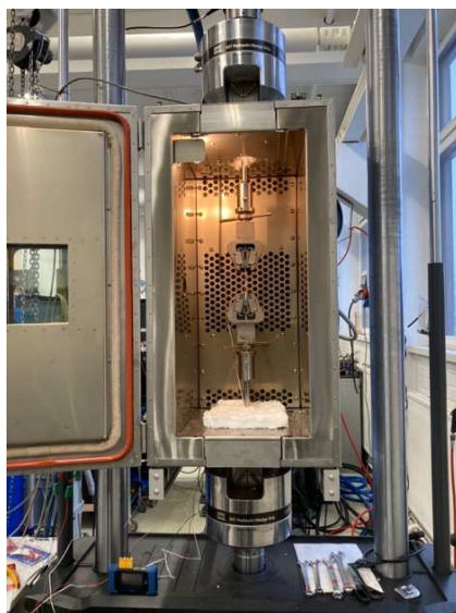
Figure 3. The chamber used for tensile testing in low and high temperatures at 1 atm.
