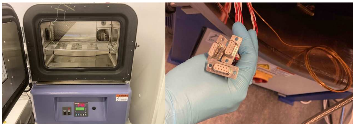
Figure 5. The Espec® chamber for temperature cycling in 1 atm. (left picture), and electrical and data connectors available inside the Aalto Spacelab's thermal vacuum chamber (right picture).
