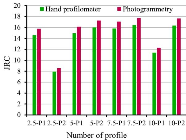
**Figure 7.** Difference between JRC values obtained from manual profilometer and photogrammetric method, for the upper joint surface and at the sampling step of 1.27 mm.
