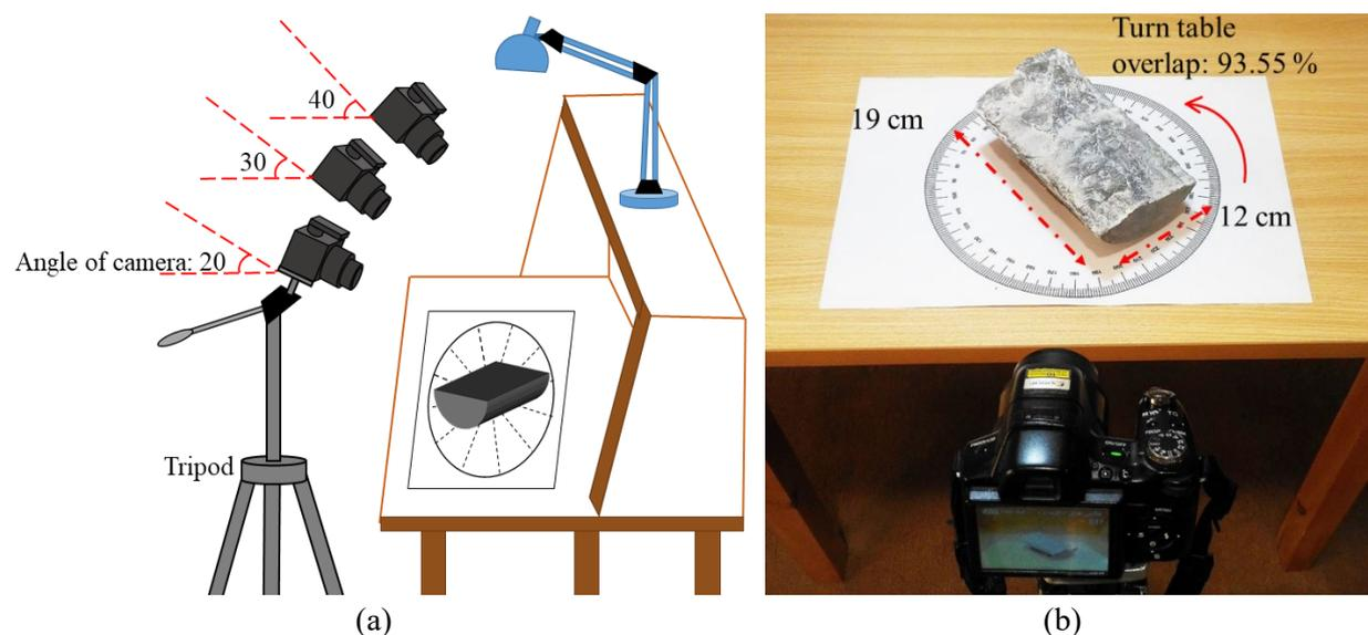
**Figure 3.** (a) Schematic diagram of photogrammetric process. (b) Sample placed on the rotating plate.
