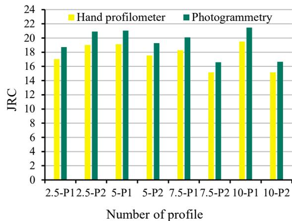
**Figure 10.** Difference between JRC values obtained from manual profilometer and photogrammetric method, for the lower joint surface and at the sampling step of 0.42 mm.
