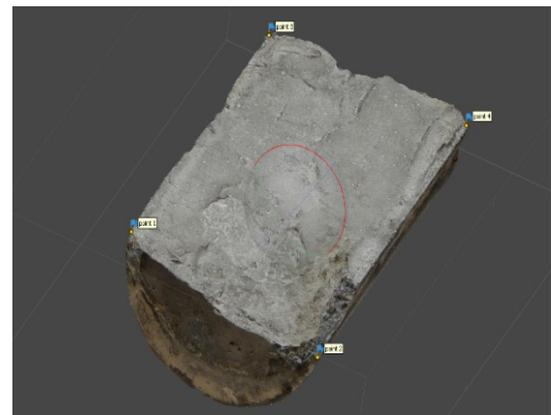
**Figure 5.** Three-dimensional model of the joint surface generated using photogrammetric process.
