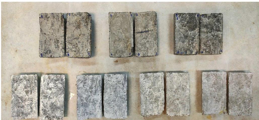
**Figure 1.** Replica samples prepared by molding from the main fracture surface.
