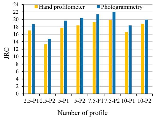
**Figure 8.** Difference between JRC values obtained from manual profilometer and photogrammetric method, for the upper joint surface and at the sampling step of 0.42 mm.
