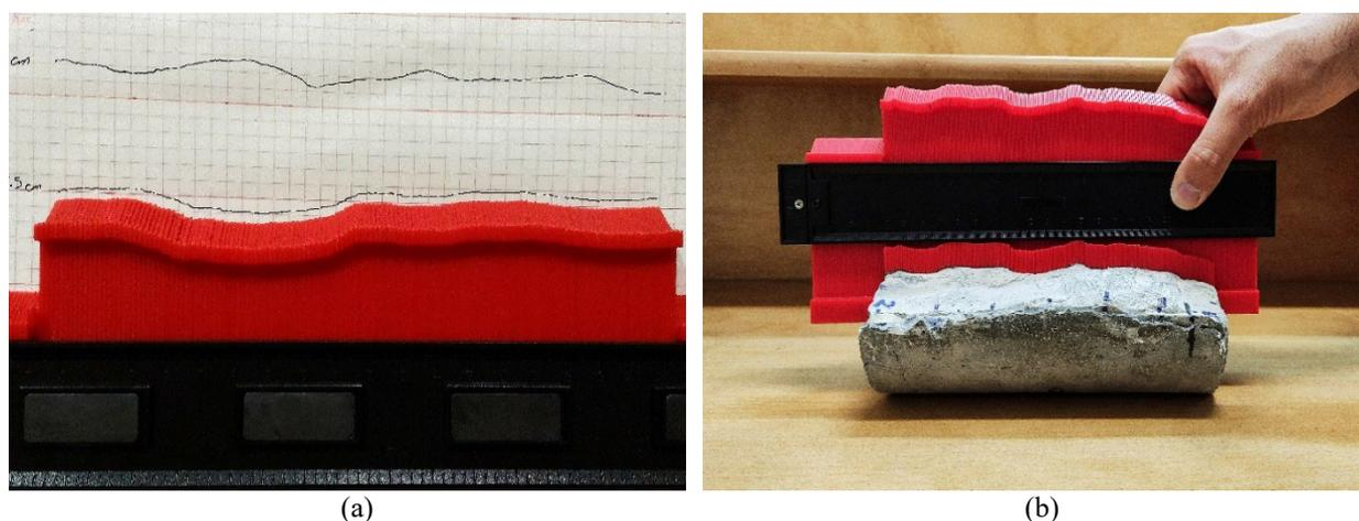
**Figure 2.** (a) Drawing the profiles of the joint A using a manual profile. (b) Positioning the profile on the joint surface so that the needles are properly placed on the surface
