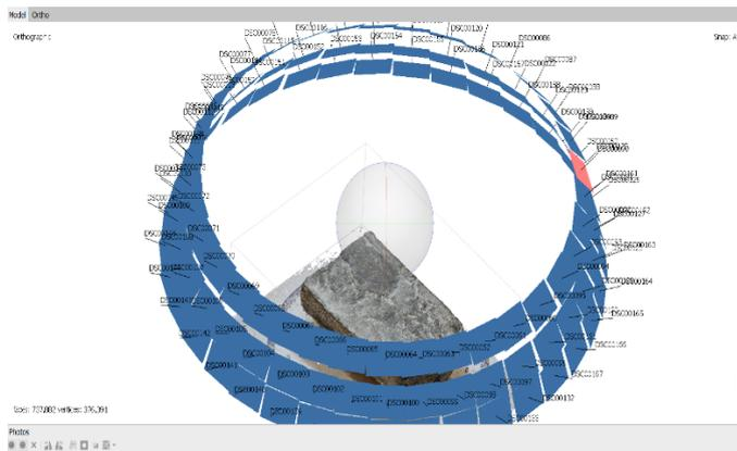
**Figure 4.** Camera positions in the photogrammetric process performed on the joint.
