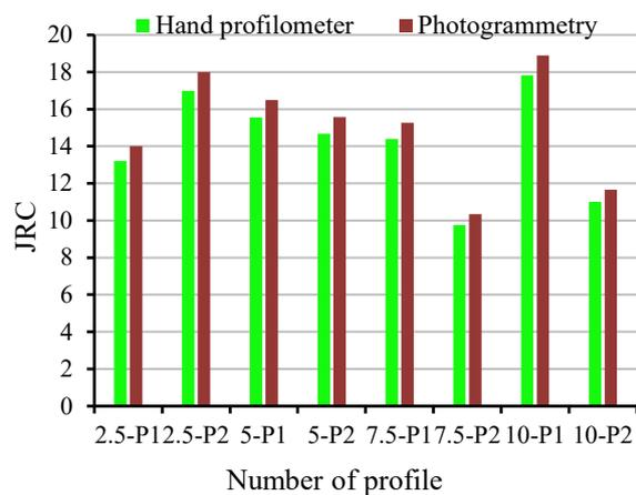
**Figure 9.** Difference between JRC values obtained from manual profilometer and photogrammetric method, the lower joint surface and at the sampling step of 1.27 mm.
