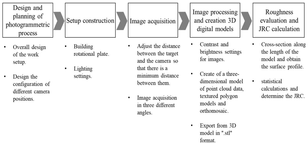
**Figure 6.** The process of calculating the joint roughness coefficient using three-dimensional models obtained from the photogrammetric process.
