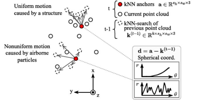
Fig. 2. The Temporal-kNN-kernel capturing temporal information. Distributions given by  $\mathbf{d} = \mathbf{a} - \mathbf{k}^{(t-1)}$ , in the spherical coordinate system, are smoother for a set of points with a uniform motion. On the contrary, a set of points caused by a nonuniform motion are more random.
