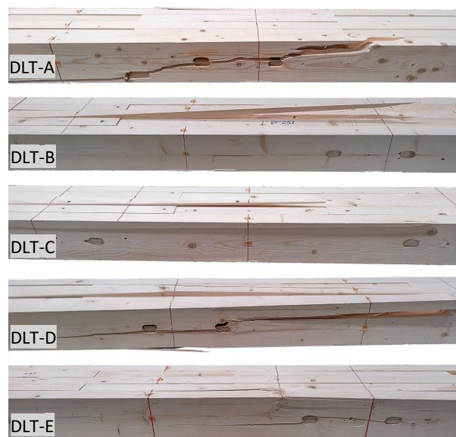
Figure 8. Failure modes of the large-scale DLT panels (view of the bottom surface of the panels).
