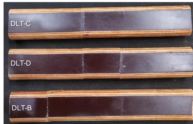
Figure 9. Shear deformations in the salvaged plywood tenons.
