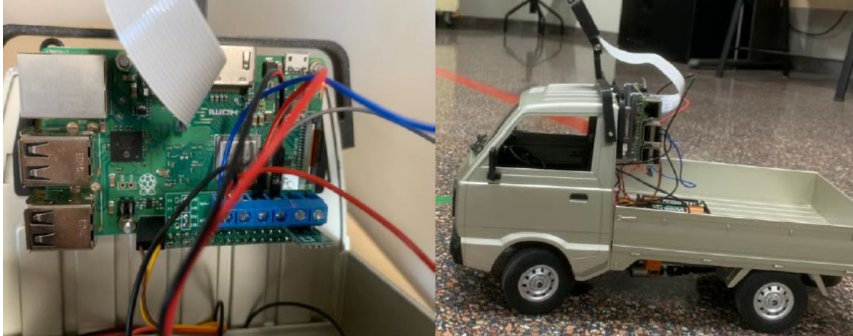
Fig. 1. Van vehicle adapted with Raspberry Pi 3 B+.
