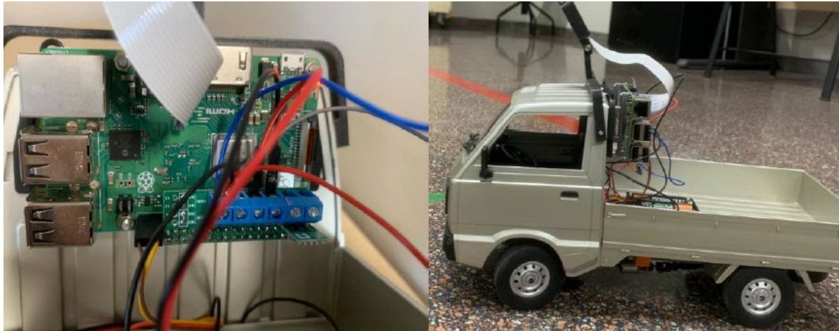
Fig. 1. Van vehicle adapted with Raspberry Pi 3 B+.
